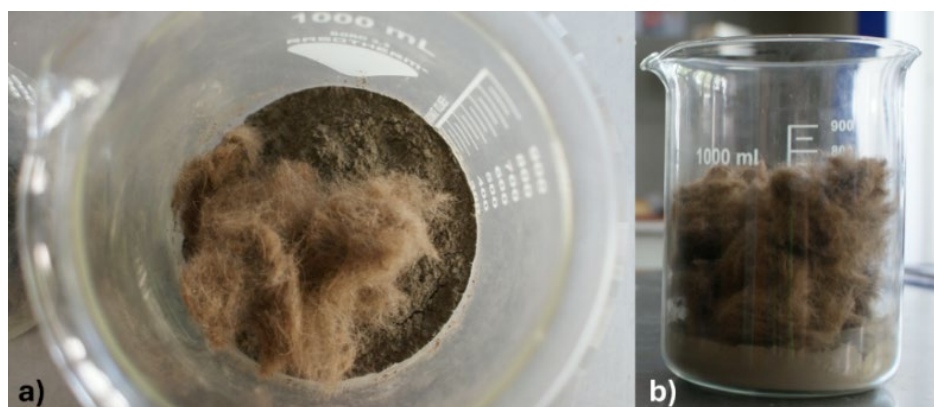
Figure 1: Solid dry ingredients: FA milled at the bottom of the beaker, with a) 1 m%, and b) 5 m% of CBR fibres on top.
