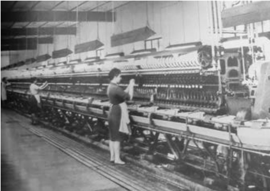
Modern equipment for reeling silk cocoons into yarn in a factory in Murcia, 1970 (Source / F. C. González)
