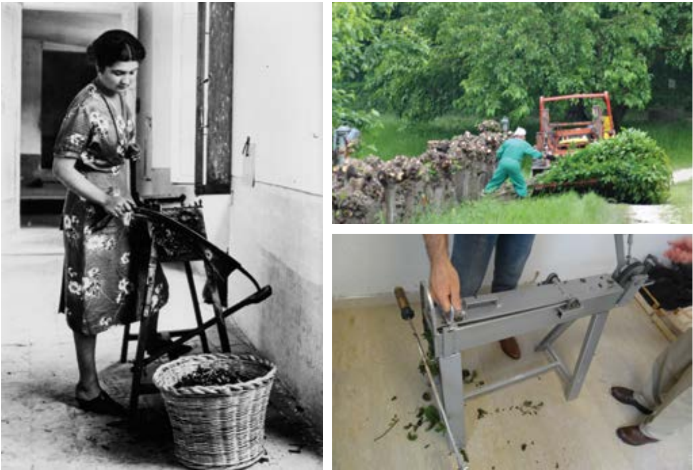
Photo top left: A photograph of a woman using a leaf-cutting machine (Source / CREA Sericulture laboratory) Photo top right: Mulberry shoots are harvested from mulberry trees which form a fence. These mulberry trees are pruned and trained using a special technique called pollarding (Photo / A. Urbanek Krajnc) Photo bottom right: Modern version of a leaf-cutting machine made of metal (Photo / A. Urbanek Krajnc)
