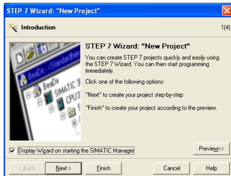
Figure 15.26: STEP 7 Wizard for creating a New Project
