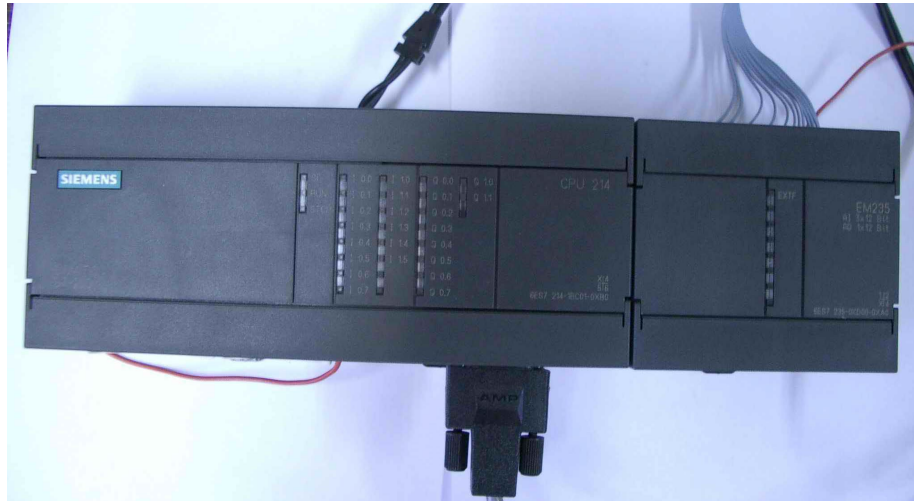
Figure 7.1: Laboratory control system based on PLC CPU 214 and EM 235 modules
