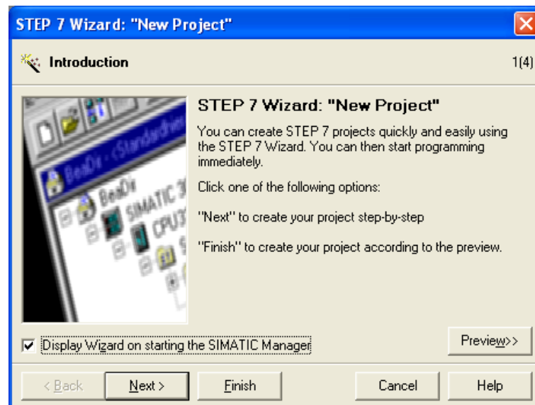
Figure 15.12: STEP 7 Wizard for creating a New Project
