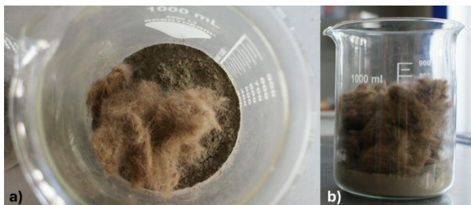
Figure 1: Solid dry ingredients: \text{FA}_{\text{milled}} at the bottom of the beaker, with a) 1 m%, and b) 5 m% of CBR fibres on top.
