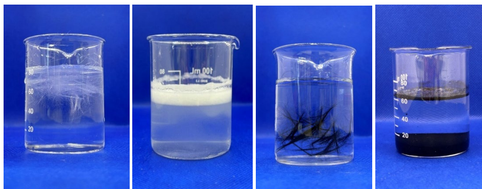
Figure 3: Sink-float method for (micro)fibrils (from left to right: f-PP, μf-PP, f-rPET, μf-rPET).
