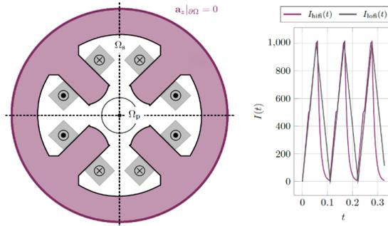
**Fig. 1.** Left: Schematic of the quadrupole magnet, where  $\Omega_{\text{Fe}}$  denotes the domain of the iron yoke,  $\Omega_{\text{s}}$  the domain of current excitation and  $\Omega_{\text{p}}$  the aperture domain. Right: Current excitation  $I_{\text{hifi}}$  for the high-fidelity model and  $I_{\text{lofi}}$  for the low-fidelity model.
