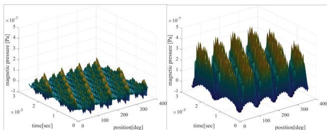
**Figure 6: Magnetic stress difference with respect to three-phase winding: a) for six-phase winding, b) for nine-phase winding**
