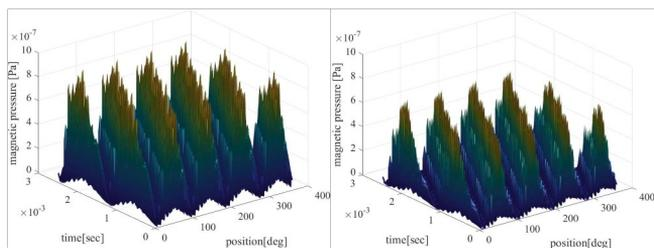
**Figure 5: Spatial-time characteristics of magnetic stresses: a) three-phase winding, b) nine-phase winding**
