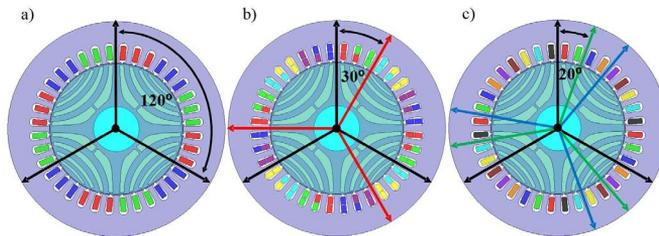
**Figure 3: Model configurations: a) three-phase, b) six-phase, c) nine-phase**
