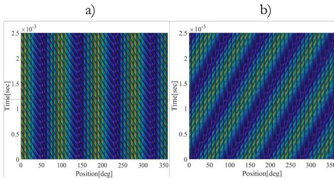
**Figure 4: Differences in the perception of radial forces depending on the reference point: a) rotor reference, b) stator reference**
