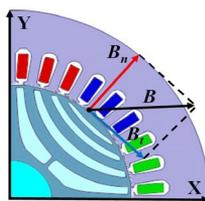
Figure 1: The components of magnetic flux density in the machine
