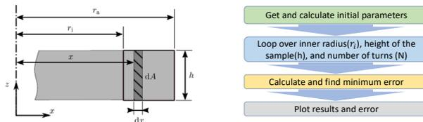
Figure 2: Ring-shaped specimen (left), optimization flowchart (right)
