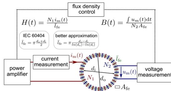
Figure 1: Experimental setup for characterizing soft magnetic materials with a ring-shaped specimen, taken from[6].
