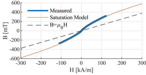
Figure 1: Measured BH curve of specimen 1
