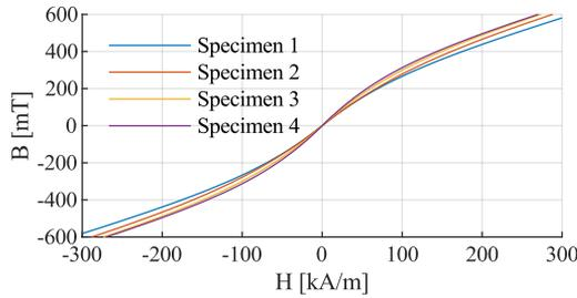
Figure 2: Fitted BH curves of the four specimens
