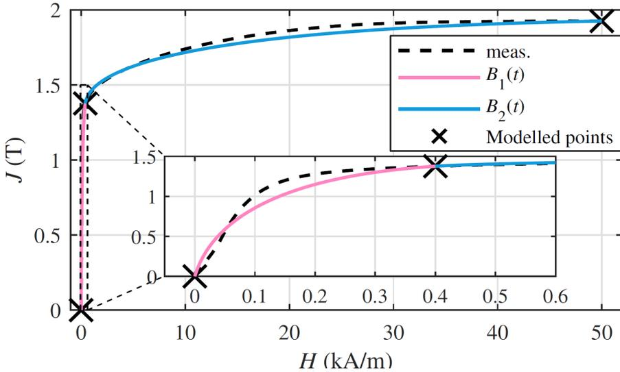
Figure 2: Modelled anhysteretic curve of a NO27 steel sheet with two joint second order Bézier curves.
