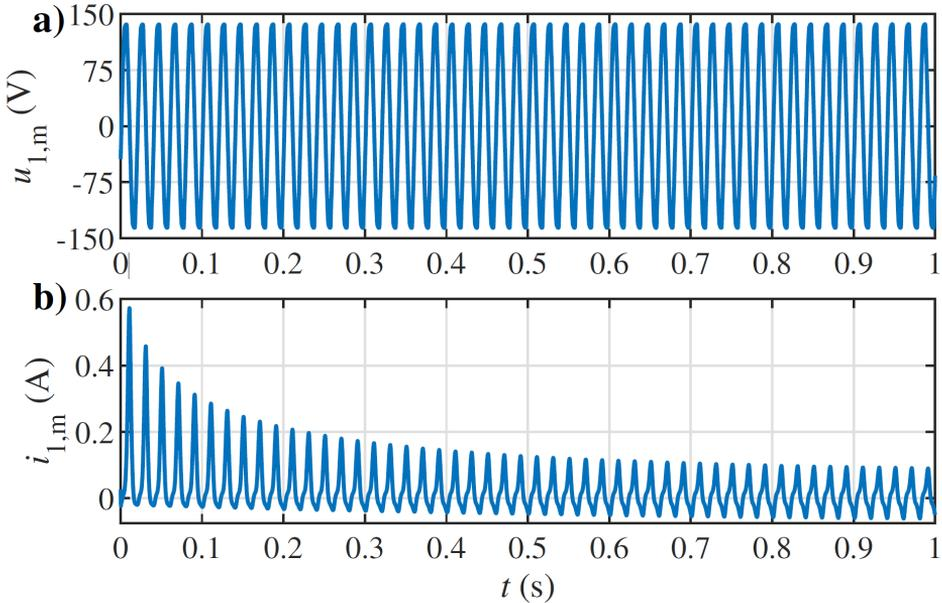
**Figure 1: a) Measured primary voltage  $u_{1,m}$  and b) measured primary current  $i_{1,m}$ .**
