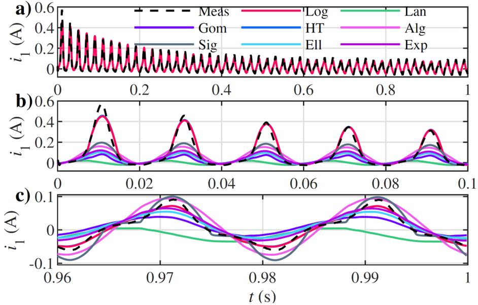
Figure 2: a) Measured current  $i_{1,m}$  and current  $i_1$  calculated with the Logistic function, b)  $i_{1,m}$  and  $i_1$  of all analytic functions in the first five periods and c)  $i_{1,m}$  and  $i_1$  of all analytic functions in the steady state.
