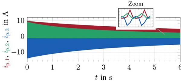
Figure 7: simulated inrush current of the three-phase transformer
