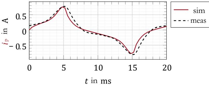
Figure 3: comparison between the simulated and measured idle current of the single-phase transformer in steady-state
