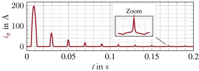
Figure 4: simulated inrush current of the single-phase transformer
