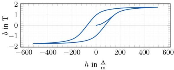
Figure 5: simulated hysteresis of the single-phase transformer
