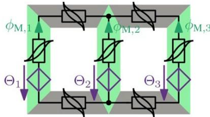
Figure 2: magnetic network of the three-phase transformer
