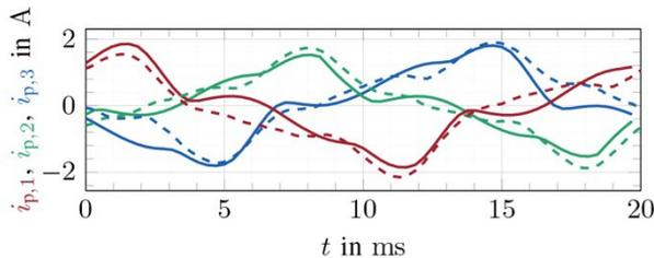
Figure 6: comparison between the simulated and measured idle current of the three-phase transformer in steady-state
