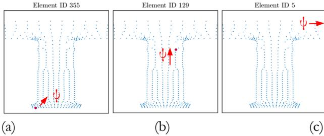
Figure 3: Selected mesh elements under investigations in three representative positions: (a) tooth end, (b) tooth center, (c) back-iron.
