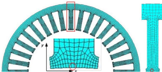
**Figure 1: Selected symmetrical domain of FEM calculation, a tooth mesh of finite elements with selected single element, and defined coordinate system.**
