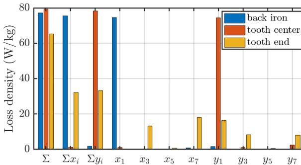
Figure 4: Components of iron loss density arranged by direction and higher harmonic components in three representative mesh elements for operating point ( $I_d = -463$  A,  $I_q = 624$  A).
