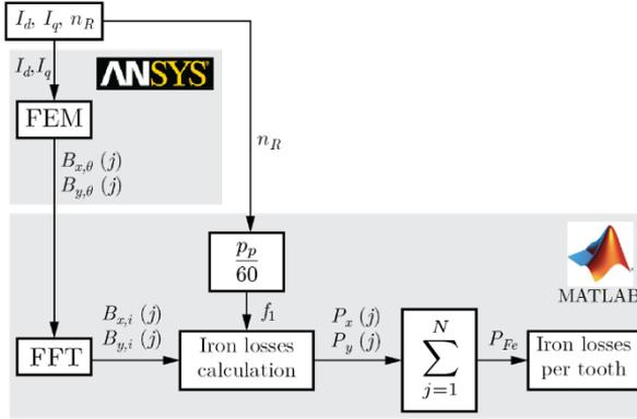
Figure 2: Flow chart of iron loss density calculation in one stator tooth for a chosen rotor speed and a single load operating point.
