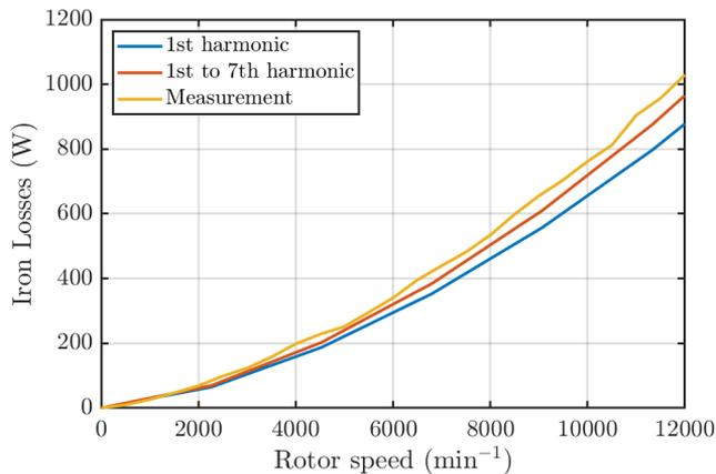
**Figure 5: Improved calculation of PMSM iron losses taking into account also corresponding higher harmonics of  $B_x$  and  $B_y$  for a wide speed range.**
