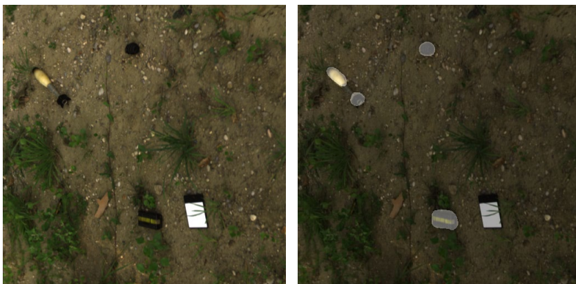
Figure 3: Example of successful UXO detection with the M3 model: original RGB image (left) and model prediction overlaid on the RGB image (right).
