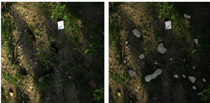
Figure 4: Example of unsuccessful UXO detection with the M3 model: original RGB image (left) and model prediction overlaid on the RGB image (right).
