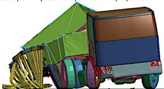
Computer simulation of a 38-ton truck hitting a road safety fence
