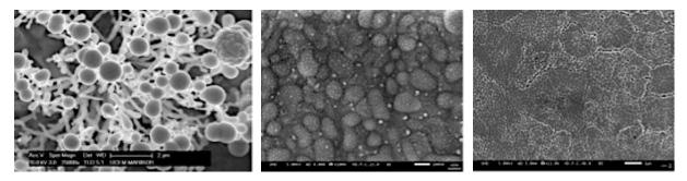
The images show nanoparticles and the microstructure of a high-entropy alloy from the Ag-Pt-Pd-Cu-Ni system after rapid solidification.
