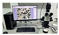
**Stereomicroscope Olympus** *SZ10* **with EP50 camera Olympus** Magnifications from 6.3x to 63x.
