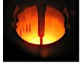
Melting in a vacuum induction furnace
