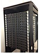
**HPC CORE@UM** is a micro supercomputer with 3 TERAFLOPS of computing capacity, designed to perform complex scientific computer simulations. The installed software enables the implementation of complex nonlinear simulations of the behaviour of solids and liquids and multiphysical problems for a wide range of research and industrial applications.
