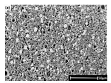
**Development of new types of filaments for 3D printing of plastomagnets** and **the development of new hybrid plastomagnets**, in which the matrix is made of TPU and PA12, and the magnetic particles of NdFeB are a combination of particles made with "melt spin" technology and gas atomisation.
