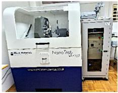
Micro- and Nanoindentation Nanotest Vantage Micro Materials Micro- and Nanoindentation Nanotest Vantage Micro Materials Force range: from a tenth of an mN to 30 N Macrohardness: from 2 N to 30 kN
