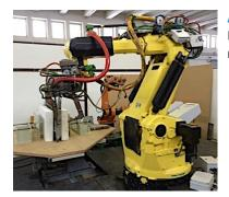
ACMA XR701 ABB Ltd Basic specifications: freedom levels: 6, load capacity: 160 kg, reach: 2800 mm, repeatability: ± 0.3 mm.
