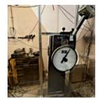
The instrumented Charpy pendulum Amsler RPK 300 with its own Vuhi-Charpy 2024-ver1 program, is intended for an in-depth study of impact testing, where the total fracture energy can be determined, which is divided into crack formation energy and crack propagation energy. Also determined are the behaviour of the material during the fracture itself and the percentage of tough fracture.
