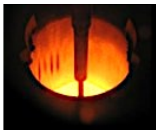
Melting in a vacuum induction furnace
