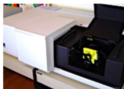
Colour samples and spectrophotometer for measurement in the U-VIS-NIR domain.
