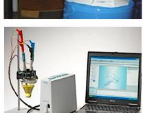
Autolab PGSTAT101 Potentiostat/Galvanostat Methrom Autolab/PGSTAT101 in combination with the powerful NOVA software is used for most standard electrochemical techniques.
