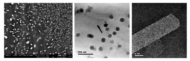
Scanning (SEM) and transmission (TEM) electron microscopy micrographs of quasicrystalline particles in aluminium alloys
