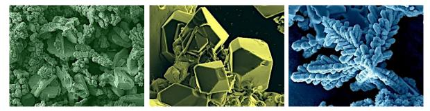
Scanning electron microscopy images of extracted phases from aluminium alloys
