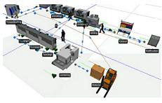
SIMIO simulation software package Simio LLC, Sewickley, USA The SIMIO package is a modern, object-oriented platform for 3D discrete event simulation with support for simulation modelling, scheduling and digital twins. It contains a library of applicationspecific templates that contain predefined objects, process logic and data schemas without the need for programming.
