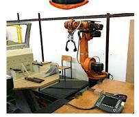
KUKA KRC1 KR15-2 Kuka AG Basic specifications: freedom levels: 6, load capacity: 15 kg, reach: 1570 mm, repeatability: ± 0.1 mm.
