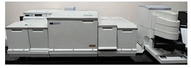
FTIR-RAMAN spectrophotometer with AUTOIMAGE microscope Perkin Elmer. Technical data: IR medium, beam splitter: KBr and Mylar, detectors: DTGS (medium IR and FIR), working range: 7000-50 cm<sup>-1</sup>, automatic imaging option, tungsten-halogen illuminator, automatic microscope. The Perkin Elmer
