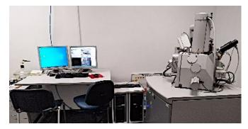
The QUANTA 200 FEI 3D Environmental Line Electron Microscope with an Ion Gun and Platinum Deposition System is an environmental electron microscope with thermal emission of electrons. The microscope allows you to work at different pressures and at 100% humidity. The environmental mode of operation – ESEM, is suitable for the analysis and characterisation of non-conductive samples (polymeric materials, ceramics, non-conductive surface layers, biological and medical preparations, etc.), and is
