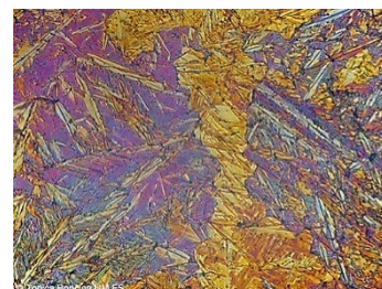
Martensitic structure of steel, colour etching and light microscopy
