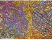
Martensitic structure of steel, colour etching and light microscopy
