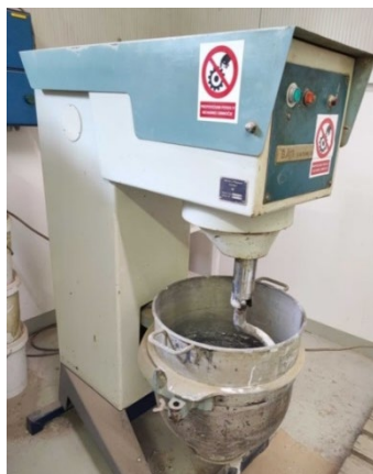
Figure 1: Mixer for the production of mixes selected for the production of pavements slabs (wet mix).
