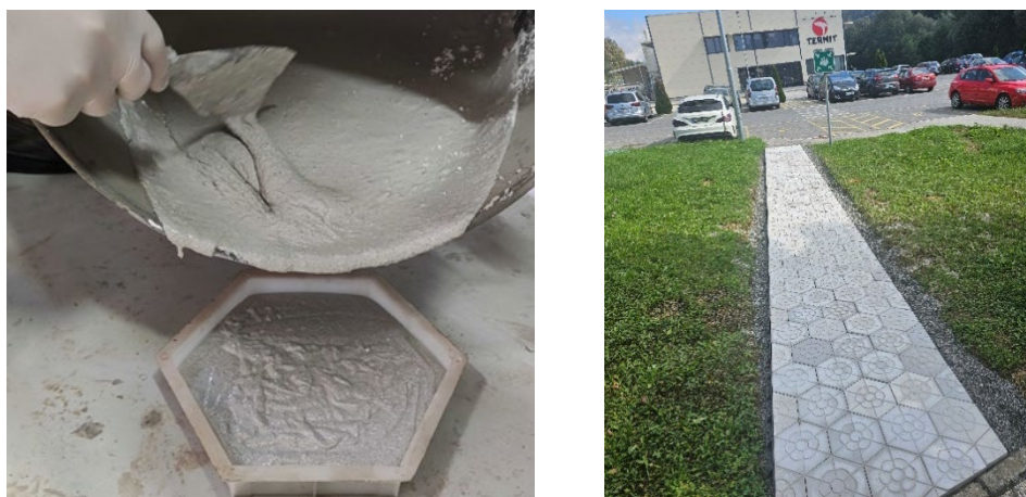
Figure 7: Filling the molds with the mixture AU (left) and testing field in the company Termit d.d. (right).
