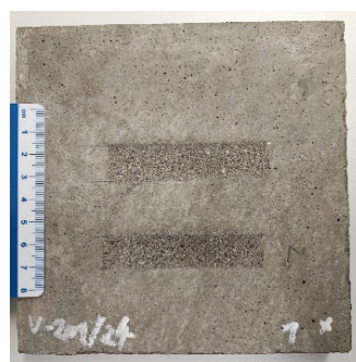
Figure 3: Evaluating freeze-thaw resistance through resonant frequency measurements with a Grindosonic after n-cycles (left); samples after abrasion resistance testing (right).
