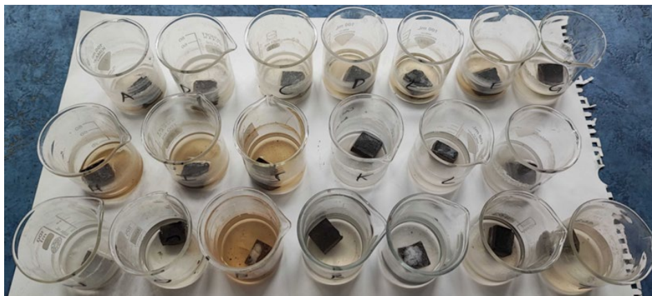
Figure 4: Various samples were placed in water to test the initial water resistance of the prepared samples.
