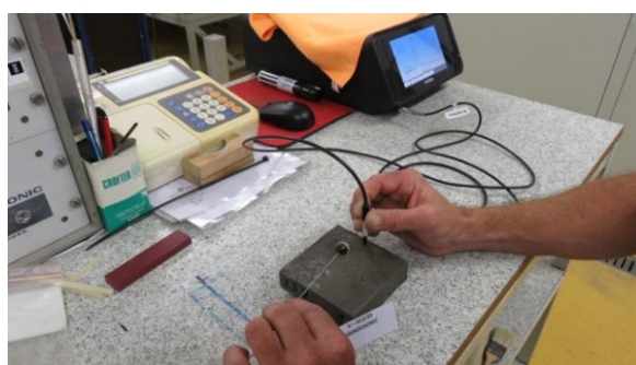
Figure 3: Evaluating freeze-thaw resistance through resonant frequency measurements with a GrindoSonic after n-cycles (left); samples after abrasion resistance testing (right).
