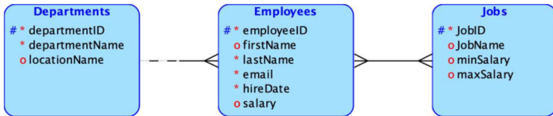
Figure 2.2: Logical Model of our Running HR Example using an ER-Diagram.
