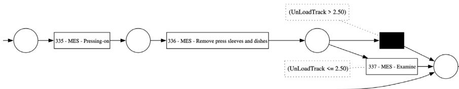
Figure 3: Example of an annotated decision point for an optional examination step in the Petri net for the most common wheelset type
