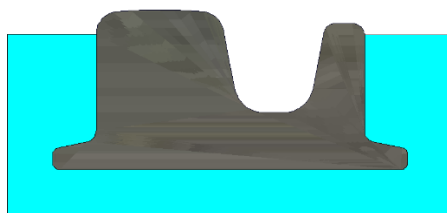
Figure 5: Finite element model of the block rail structure Source: Axis VM program
