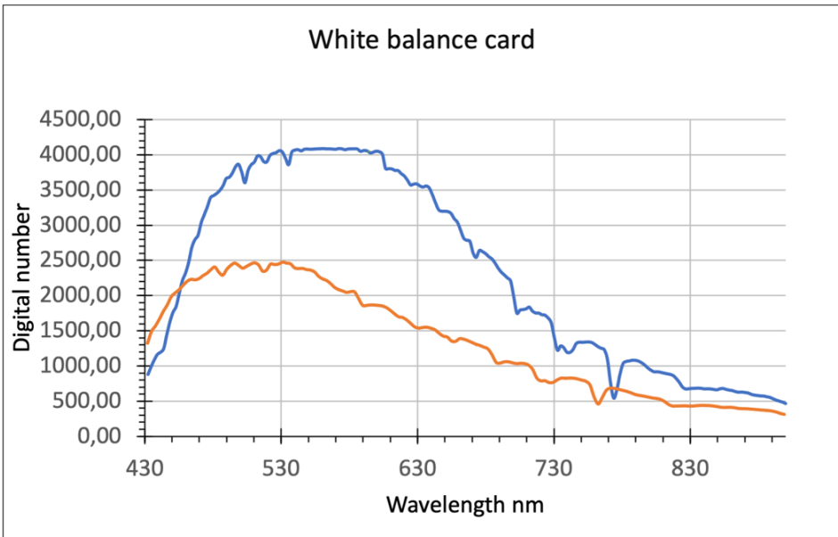
Figure 4: Uncalibrated outputs of Specim IQ (orange) and Specim Inspector V9 (blue) hyperspectral cameras by measuring the white balance card.
