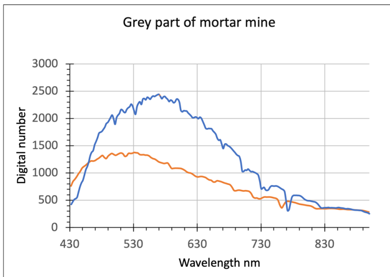
Figure 6: Uncalibrated outputs of Specim IQ (orange) and Specim Inspector V9 (blue) hyperspectral cameras by measuring the grey part of the mortar mine
