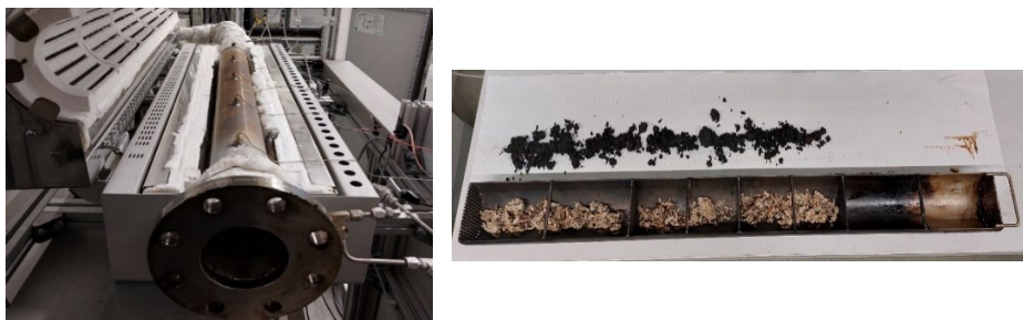
Figure 1: a) Carbolite tube furnace b) The tray with material
