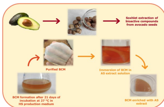
Figure 1: Procedure of production and enrichment of BCMs with AS extract Source: own.
