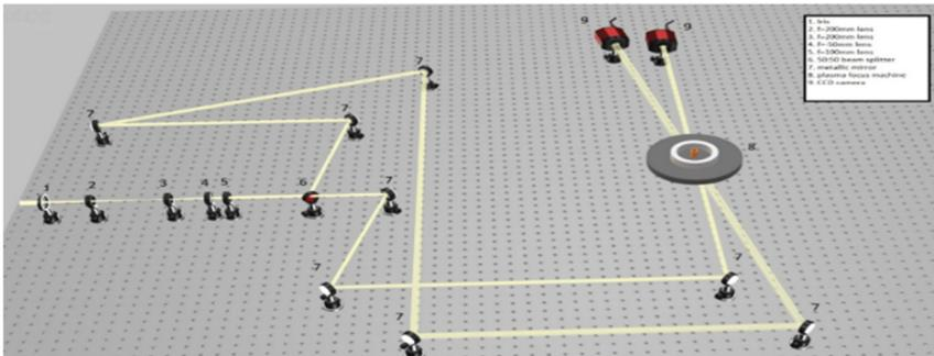
**Figure 3.** Schematic representation of the shadowgraphy setup
