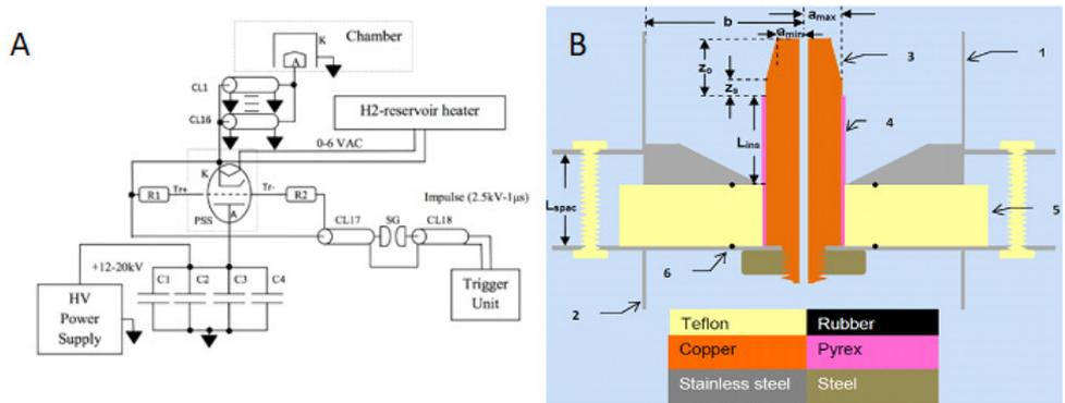
**Figure 1.** A. Electric circuit of the old version of the machine. B. A full sectional side view of the vacuum chamber. 1. Part of the chamber tube (cathode), 2. Part of the chamber tube (anode), 3. Main electrode of the anode (hollow cylinder), 4. Insulator sleeve, 5. Electrical insulation spacer, 6. O-ring for maintaining the vacuum.
