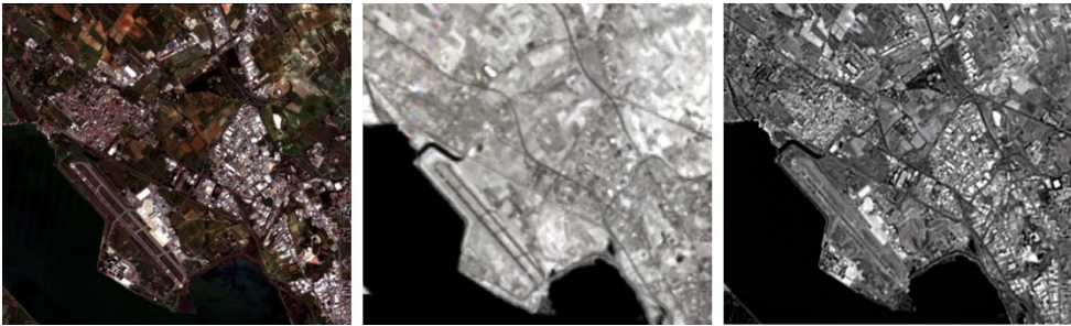
Figure 2. Left Sentinel-2 image, centre PRISMA image, right HS super resolution (SR) image
