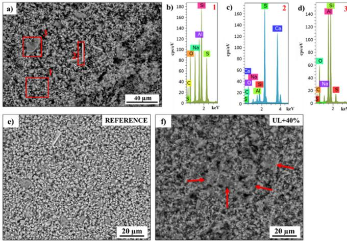
**Figure 1.** SEM micrographs in BSE mode and EDS spectra. (a) micrograph of ultramarine blue pigment; (b-d) EDS spectra of ultramarine blue pigment, (e) micrograph of the not-irradiated area, (f) micrograph of the surface irradiated at the highest fluence with Nd:YAG at 1064 nm; red arrows indicate crust melting.
