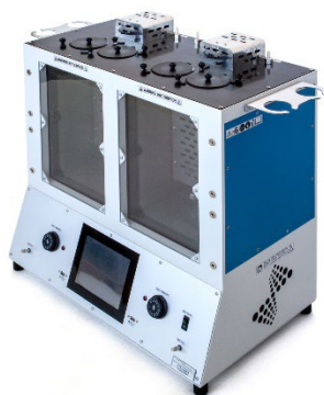
Figure 3: Device for determining foaming properties of lubricating oils.
