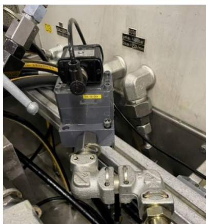
Figure 6: Flow meter mounted on the rail in front side of the test bench.
