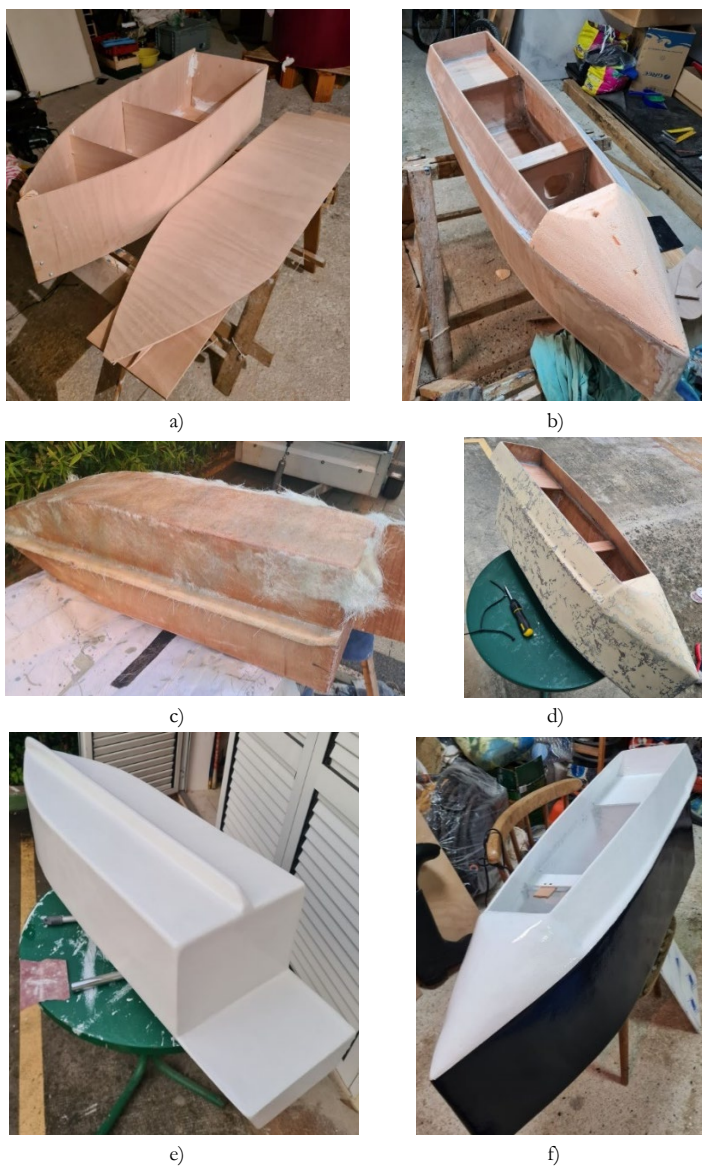
Figure 2: Stages of boat hull construction, a) screw connection, b) polyester binding, c) plasticizing, d) coating with cement kit, e) primer coating, f) coating with final paint
