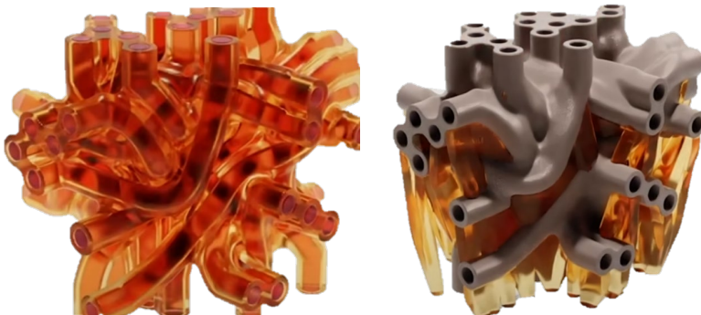
Figure 13: Hydraulic block optimized to achieve minimum mass requirement.
