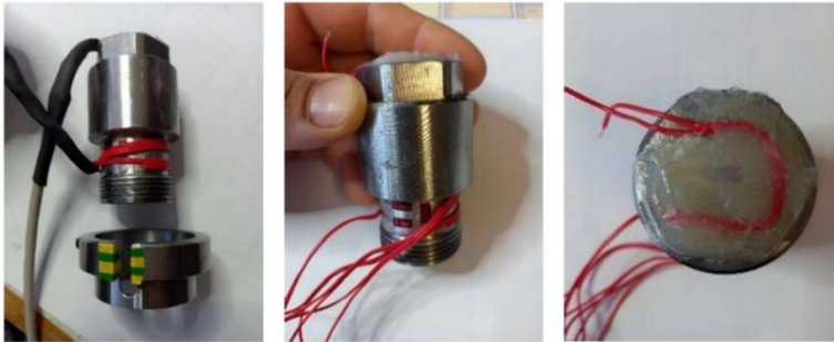
Figure 9: Modified plug M33x2 equipped with strain gauges Source: own
