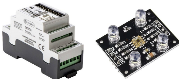
Figure 11: PLC Controllino Mini and color sensor TAOS TCS3200.
