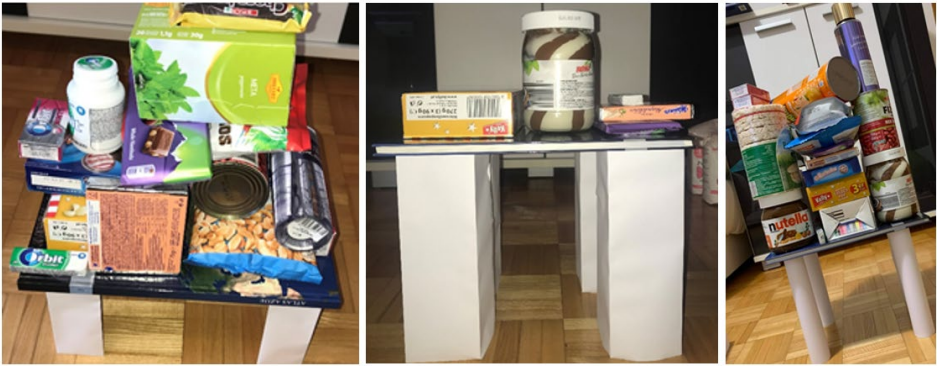
Figure 2: Example of testing the strength of paper profile legs
