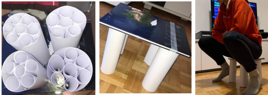
Figure 3: Example of constructing and testing paper chair legs
