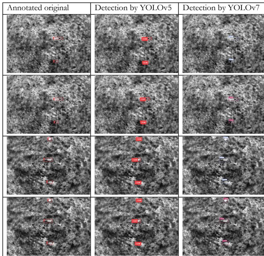
Figure 3: Qualitative results for the single UXO class detection problem: Expert annotations are overlaid on the thermal images (left column) and bounding boxes with UXOs, detected by using the pretrained YOLOv5n and YOLOv7 tiny (rows 1 and 3, middle and right column) or YOLOv5x and YOLOv7 regular (rows 2 and 4, middle and right column). A single class index 1 and detection probability are written next to the bounding box.
