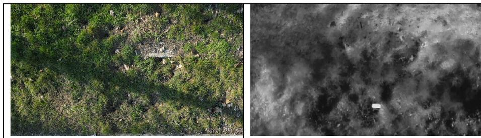
**Figure 4. A land mine with a green metal casing placed on green grass: An image in the visible spectrum (left) and the same terrain in the thermal spectrum (right). Note: This example is from our private database and is not part of the UXOTi\_NPA dataset.**
