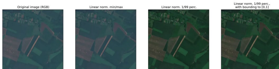
Figure 2: True color Sentinel-2 image before and after various transformations. The last image shows the transformation resulting in best model performance.
