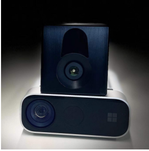
Figure 3. Integration of Monstar and Azure Kinect
