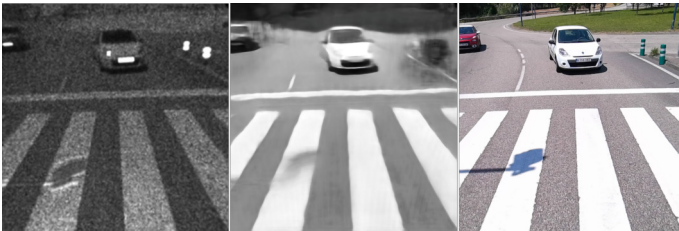
Figure 4. Left: the infrared image; Middle: the reconstructed grey image; Right: RGB image
