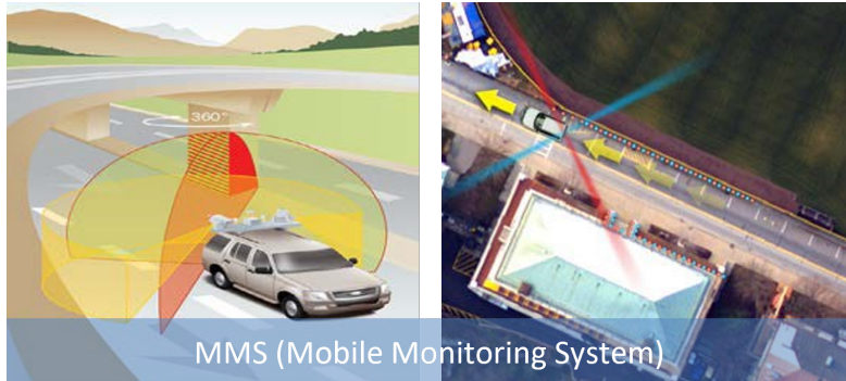
Figure 1. An example of Mobile mapping system
