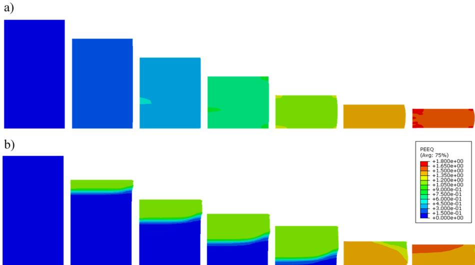
**Figure 3.** Evolution of the equivalent plastic strain (PEEQ) during the quasi-static (a) and high strain rate (b) deformation response of closed-cell foam modelled with homogenised computational model.
