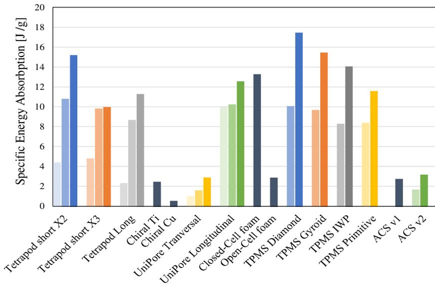
**Figure 8.** Comparison between the computational and experimental results
