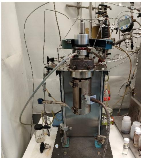
**Figure 1: 300 mL high-temperature and high-pressure reactor.**
