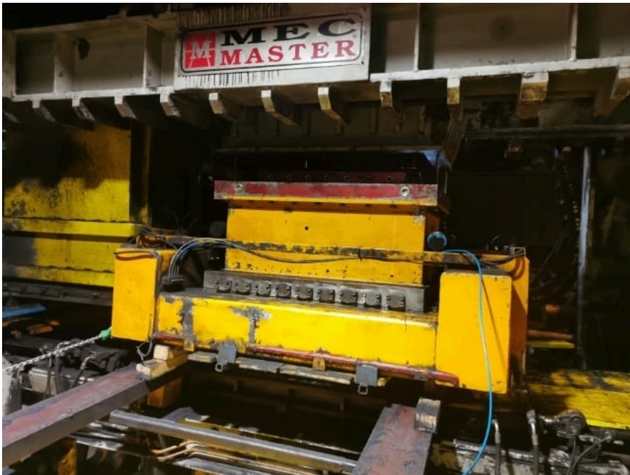
Figure 3: Physically released hydraulic block of the press.
