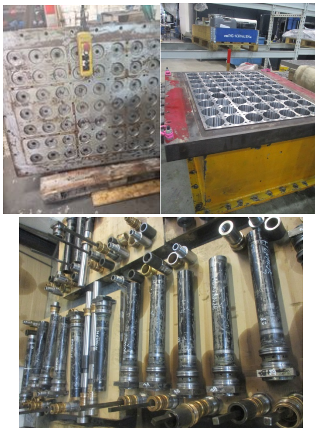
Figure 4: Disassembly of the hydraulic block into component subassemblies.
