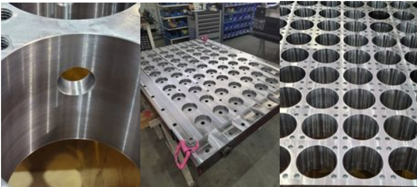
Figure 6: Cover and guide plate form roller housings
