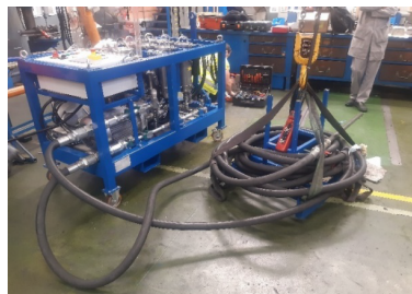
Figure 7: Carrier for hoses and hoses for suction and return line attached to the chain lift for easier transportation.
