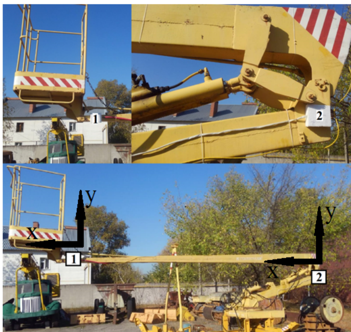
Figure 1: Points of installation of two-dimensional accelerometers.
