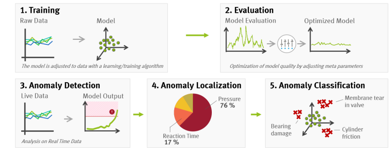
Figure 7: Anomaly detection and classification, Source: Festo SE & Co. KG.
