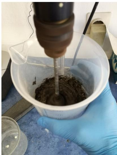
**Figure 1: Homogenization of AA pastes.**
