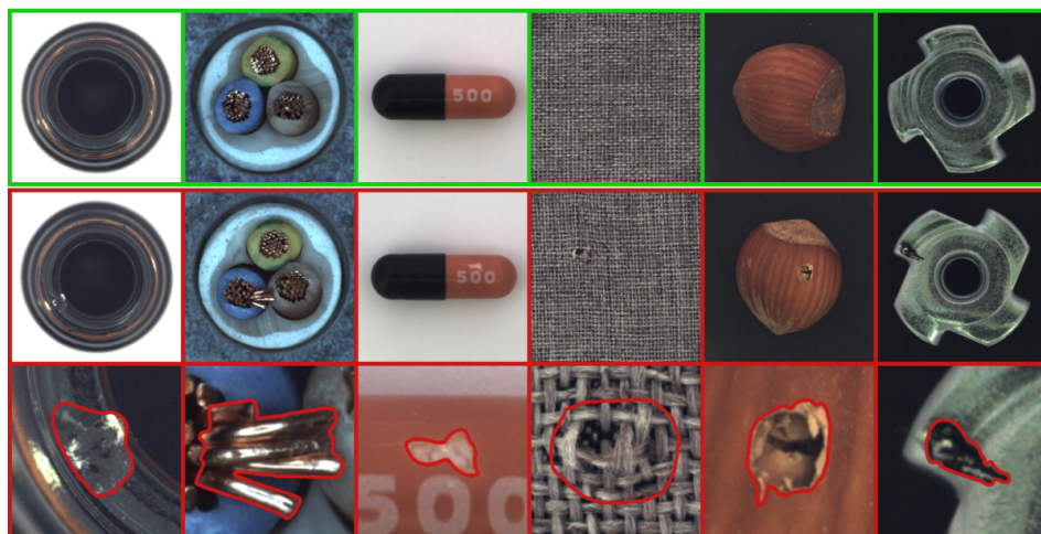
Figure 1: Samples from MVTec AD dataset [21]. First row represents normal samples from the training set (bottle, cable, capsule, carpet, hazelnut, metal nut), second row the same objects with various defects and the third row presents pixel-wise annotations for defective samples. Image adapted from [21].
