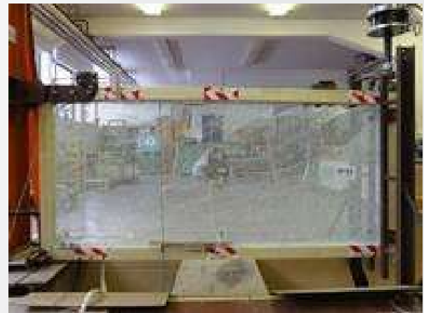
Load Bearing Timber-Glass Composites LBTGC – Racking tests
