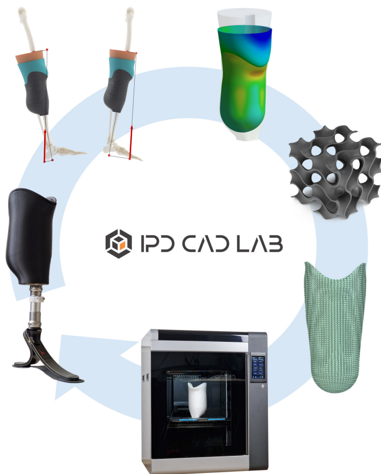
Shematski prikaz uporabe integriranega razvojnega procesa za razvoj naslednje generacije 3D-natisnjenih nožnih protez Schematic illustration of the use of an integrated development process to develop the next generation of 3D printed foot prostheses
