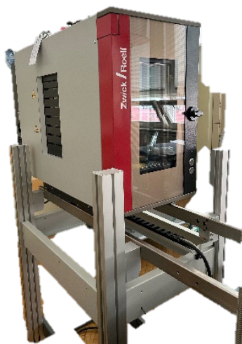
Temperaturna komora Zwick/Roel (-80 °C do +250 °C) Temperature chamber Zwick/Roel (-80 °C to +250 °C)
