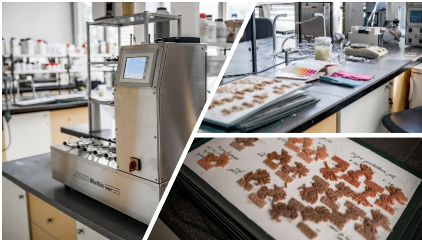
Laboratorij za barvanje in vzorci volne, obarvani z naravnimi barvili Dyeing device and wool samples dyed with natural dyes
