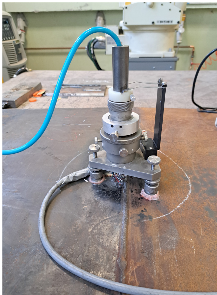
Meritve zaostalih napetosti z metodo vrtnja izvrtine na zvarnem spoju, obdelanem z eksplozijo Measurement of residual stresses by drilling a hole on an explosion-treated weld joint
