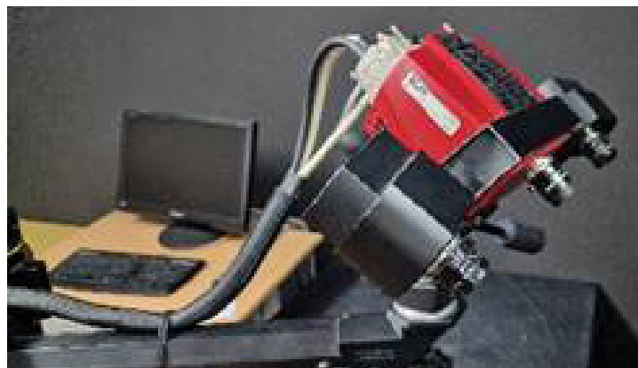
GOM Atos II 400 – 3D metrološki skener GOM Atos II 400 - 3D metrology scanner
