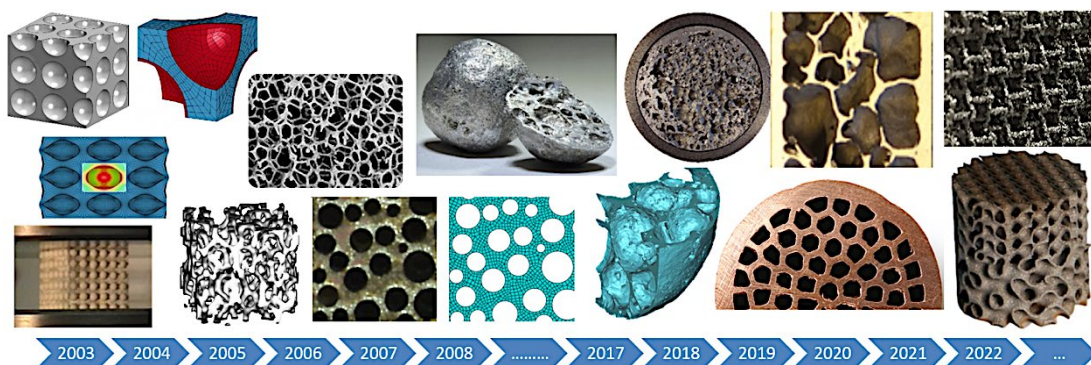
Figure 1: Research of cellular metamaterials at the University of Maribor in recent years: from primitive to advanced cellular geometries
