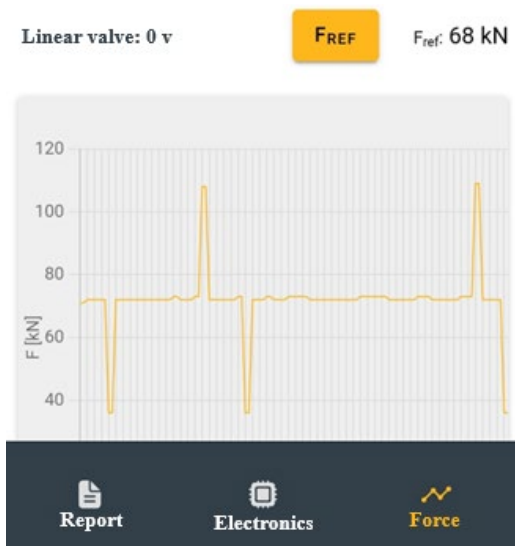
Figure 4: Recording the measured pulling force of the winch.
