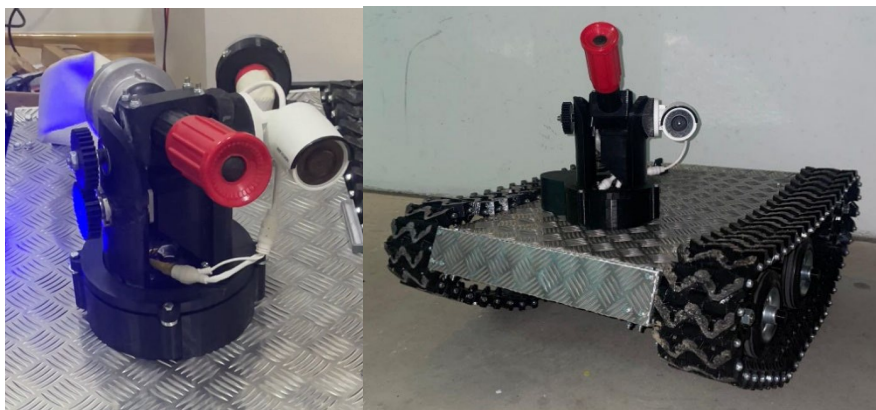
Figure 4: Mobile fire-fighting robot with mounted rotating turret.
